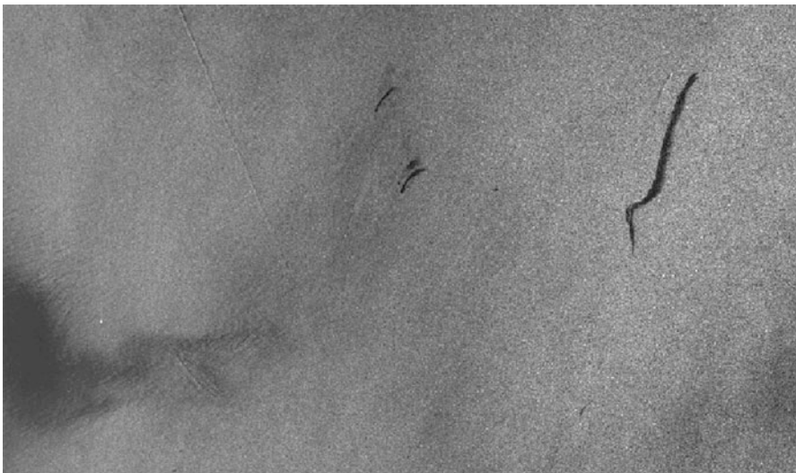
Fig. 8.2 A radar image of a sea surface. The “wiggly” elongated dark region in the upper-right corner represents environmental hazard: an oil spill (Kubat et al. [43])
