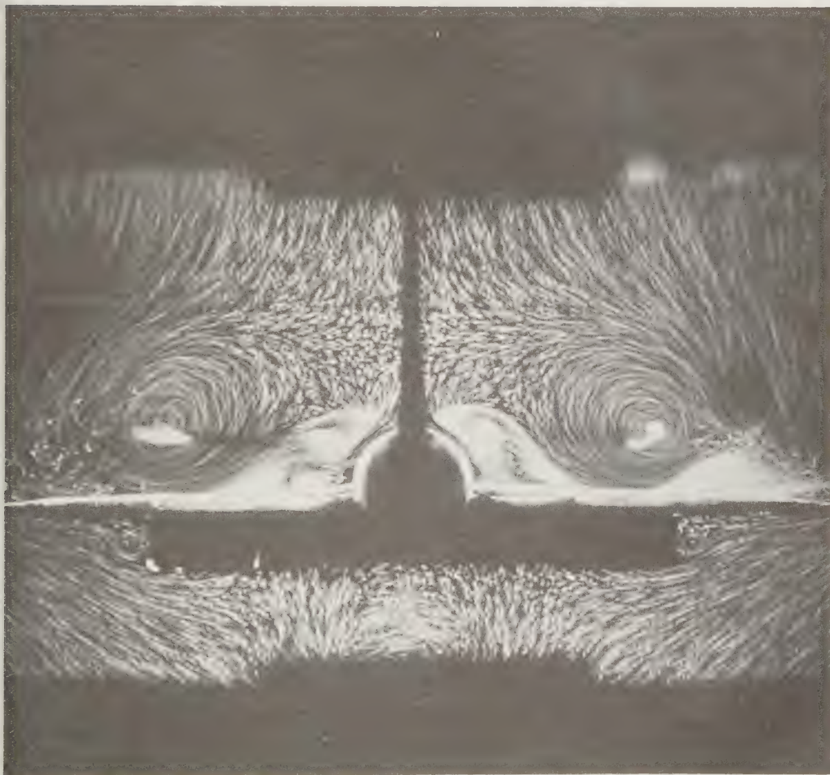
An aircraft in a hydrodynamic wind tunnel
